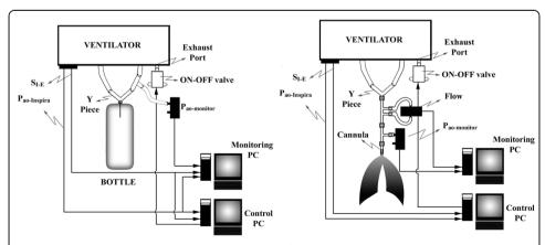
**Figure 1 Experimental set-up.** Experimental setups. Left panel: in vitro - a physical model was employed during experiments; Right panel: in vivo - here the respiratory flow was monitored.  $S_{I-E} = logic$  signal that identifies the inspiratory as well as the expiratory cycles;  $P_{ao} = airways$  opening pressure; The ON-OFF valve is the valve employed to control the PEEP.
