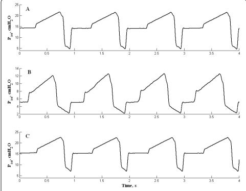
**Figure 2 Airways opening pressure waveforms.** a) The airways opening pressure  $(P_{ao})$  for a target PEEP of 5 cmH<sub>2</sub>O controlled by PEEP-old method; b) and c) The  $P_{ao}$  for the targets PEEP of 5 and 15 cmH<sub>2</sub>O, respectively, controlled by PEEP-new method. Note that for a target PEEP of 5 cmH<sub>2</sub>O the PEEP-new closes at a  $P_{ao}$  around 2 cmH<sub>2</sub>O.
