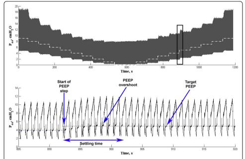
**Figure 3** Airways opening pressure during PEEP step change test. Upper panel: airways opening pressure ( $P_{ao}$ ) during the entire PEEP step change test with PEEP-new during one in vivo experiment. The dashed white lines are the target PEEP. Lower panel: detail of  $P_{ao}$  during the PEEP step change from 4 to 5 cmH<sub>2</sub>O. For this step, the arrows indicate the start of the PEEP step, the settling time, the overshoot and the target PEEP.
