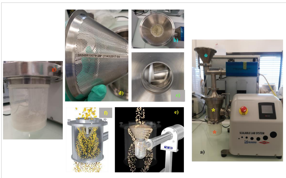
Figure 127. a) General view of Quadro® Comill with HE High energy Mill, b) material feed, c) feed screw, d) grinder, e, and f) different view of particle grinding, and g) collector. Source: Author and from [349].
