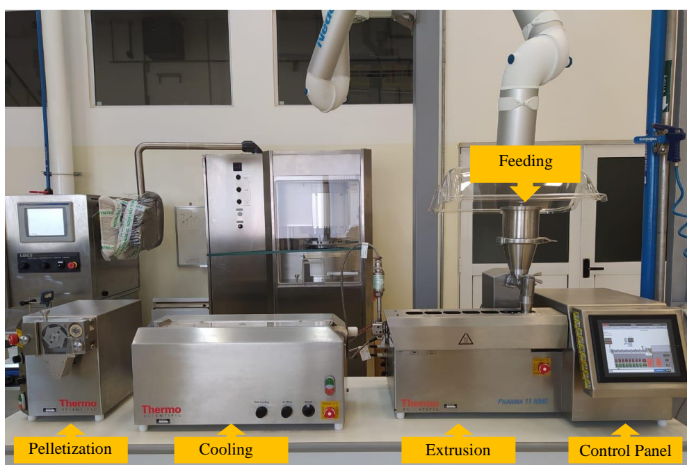
Figure 78. Extrusion system using Pharma 11 extruder.
