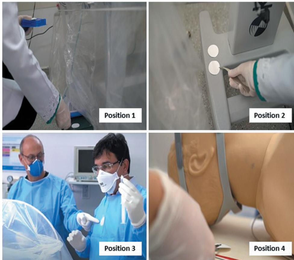
**Figure 2.** Positioning of nitrocellulose sensor discs. Position 1: entrance of multiparameter patient monitoring cables and respiratory tubes; position 2: entrance of intravenous therapy tube; position 3: on a health professional's chest; position 4: inside the ISATI.
