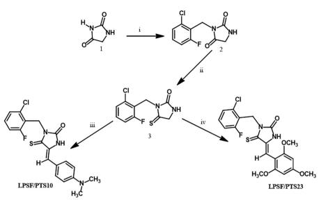
Scheme 1 - Reagents and conditions: (i) 2-chloro-6-fluorobenzyl chloride; CH<sub>3</sub>OH, NaOH, 60° C (ii) Lawesson's reagent, 90 °C (iii) 2-cyano-3-(4-dimethylaminephenyl)acrylic acid ethyl ester, CH<sub>3</sub>CH<sub>2</sub>OH, 50 °C; (iv) 2-cyano-3-(2,4,6-trimethoxy-phenyl)acrylic acid ethyl ester, CH<sub>3</sub>OH, 50 °C; (iv) 2-cyano
